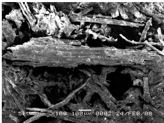
Fig. 3. SEM examination of the straw board
