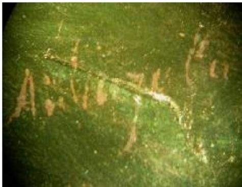
**Fig. 20 Poor adherence of the signature to the paint layer.**
