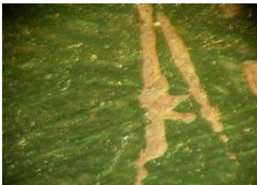
**Fig. 23The accumulation of the paint in the middle of the left side line.**
