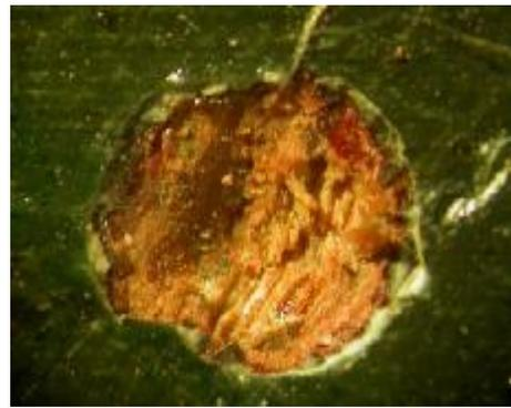
**Fig. 12** Artificial multiple dents appear as flaking.
