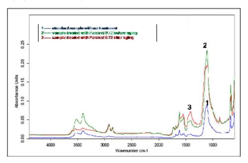
Fig. 8 shows the FTIR- ATR spectra of the sample untreated (1), treated with Paraloid B72before aging (2) and after aging (3)
