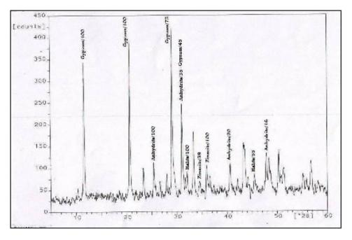
Fig. 6 the XRD patterns of the subsurface layer
