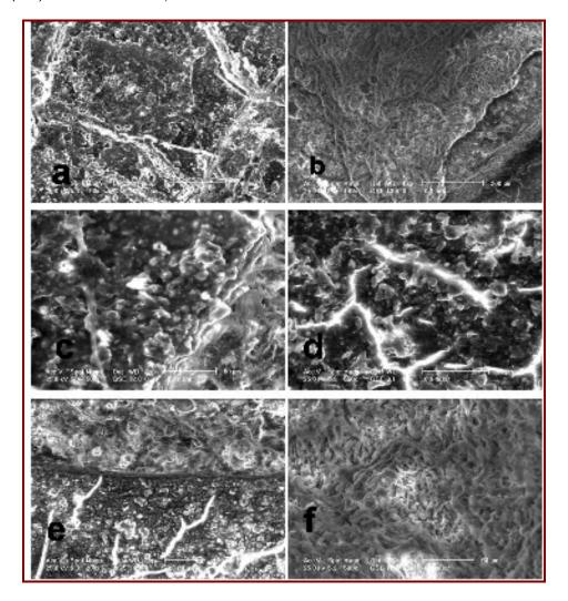
Fig.7 (a) and (c) show the SEM image of the sample treated with Paraloid B 72 before aging under different magnification, (b) and (d) show the SEM image of the sample treated with SILRES® BS OH 100 before aging. Images (e) and (f) show the SEM image of the samples treated with Paraloid B 72 and SILRES® BS OH 100 respectively.
