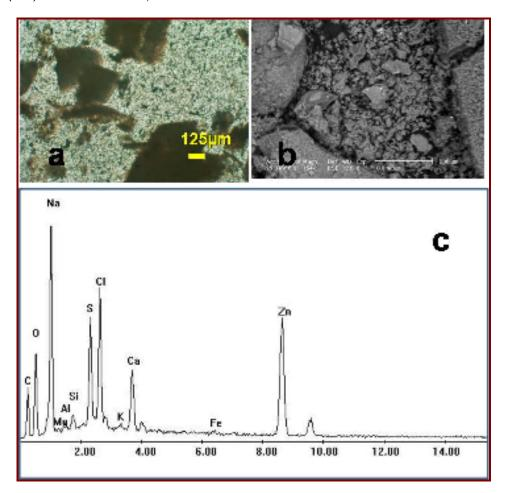
Fig. 4: (a) Photomicrograph of crushed yellow pigments in the yellow veined paint. 20X, (b) SEM image of yellow and brown grains, (c) EDX spot analysis from image (b).
