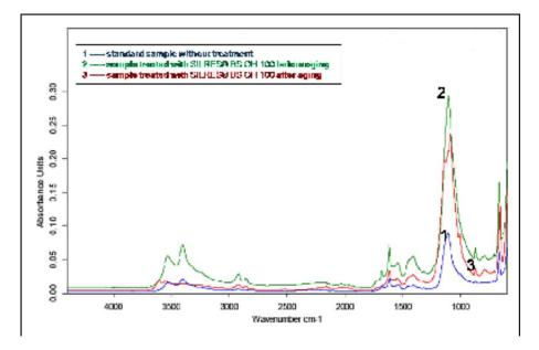
Fig. 9 shows the FTIR- ATR spectra of the sample untreated (1), treated with SILRES® BS OH 100 before aging (2) and after thermal aging (3)
