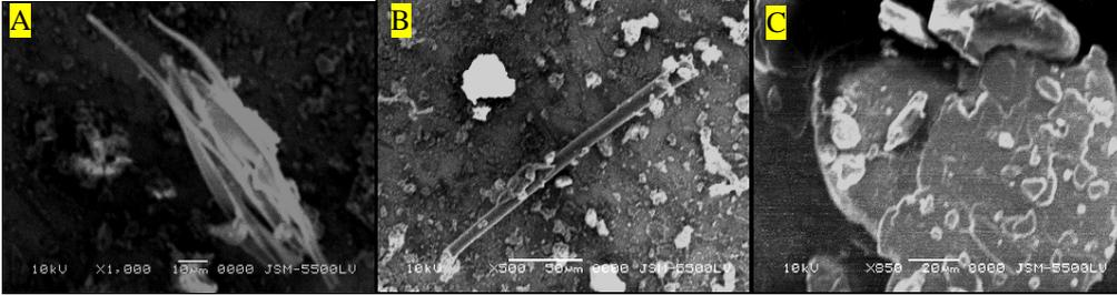
Fig.9 a-f SEM-EDX microanalysis and photomograph of limestone sample (W3) **a** growth of mite (phylum: Arthropods) **b** the algal growth **d** Exfoliation and destroyed of the calcite ooids
